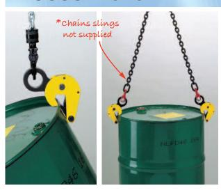
The DC500 drum clamp has been designed to lift and transport steel drums. If moving empty or sealed drums then one clamp is sufficient on its own. Should you be lifting an open full drum, then two clamps should be used with a two leg chain sling.
