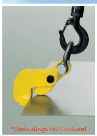
**The THK horizontal plate clamps** share the same basic design features as the CH range of clamps but have a reversed tooth jaw design. This acts as an additional safety feature specifically for use with thin sheets which may have a tendency to deflect or sag or flex.
