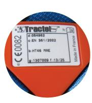
Check the date of manufacture of your Tractel harness which is located on the back plate. The life span of Tractel harnesses is 10 years from date of manufacture. If you are unsure of how to identify this on a Tractel harness, please contact Tractel for assistance.
