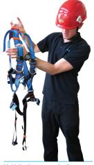
Hold the harness up by the rear 'D' and check for any twists or tangles.
